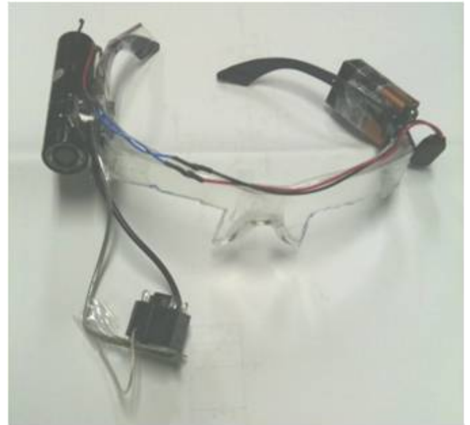
Figure 4. Low Cost Gaze Tracking Glasses. The wireless camera on the top left of the figure is what we refer to in this work as the scene camera. The scene camera approximately captures the field of view of the user. The camera on the bottom left of the figure is the gaze tracking camera that monitors the user’s gaze movements. The Haytham software uses the video stream provided by that eye camera to calculate the PoR of the user and superimposes the gaze estimation coordinates over the video stream generated by the scene camera. The top right of the figure shows the battery that is used to provide energy to the wireless cameras.
