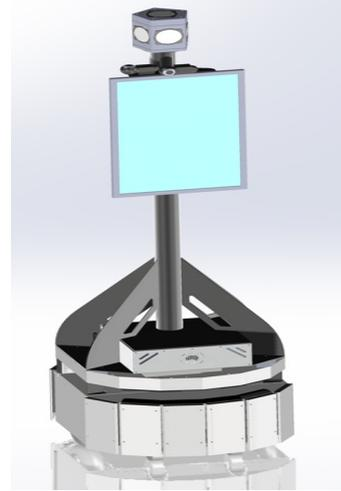
Figure 2. **Prototype of the Telepresence Robot.** The figure displays the main components of the robot, a panoramic camera on its top, a screen in the middle and a mobility unit in the bottom.
