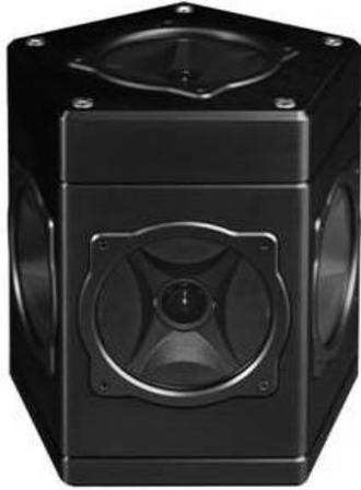
Figure 3. **Panoramic Camera.** The figure displays the Lady-Bug3 panoramic camera on top of the robot that uses several cameras facing different directions to create a panoramic image of the robot's surroundings.
