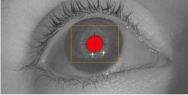
Figure 1. **The Open Source ITU Gaze Tracker Tracking One Eye.** The features being tracked in the image are the pupil center and two corneal reflections. These features are used by the gaze estimation algorithms to determine the PoR of the user on the screen.
