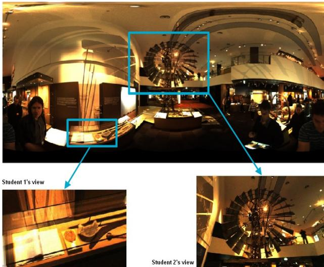
**Figure 5. Creation of an Immersive Telepresence System.** Images from the 360° camera on top of the robot are combined to form a high-resolution 2D omnidirectional image representing the environment around the robot (top image). Individual users can look at different subareas of the panoramic video stream (bottom images).
